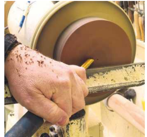
▲ Pic.3 The 10mm bowl gouge is used in a pull cut to true up the base. To keep depth of cut consistent, work from the centre out to the edge with your left hand running along the tool rest
